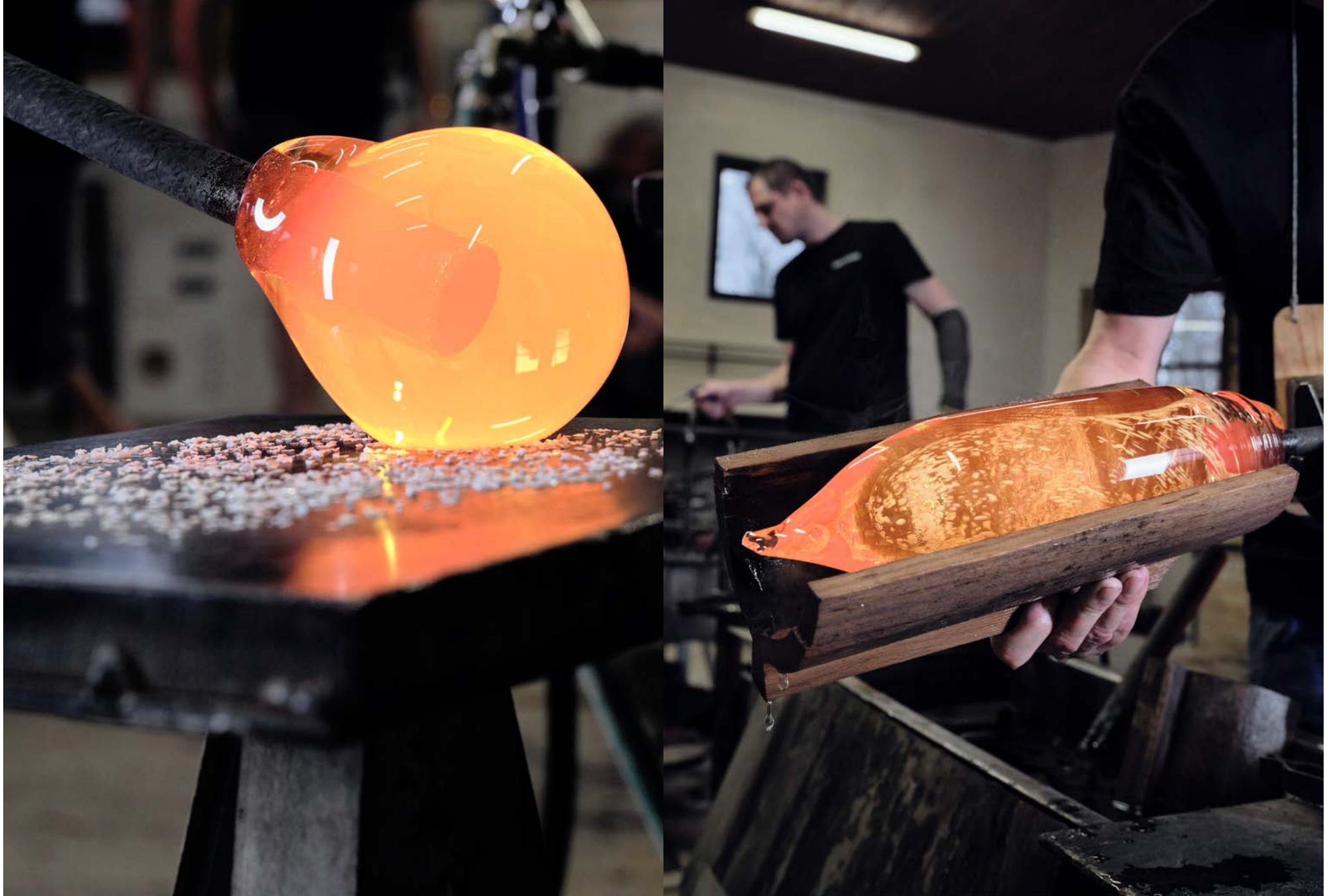
The molten-glass core is covered by small glass shards, then dipped back in molten crystal.
